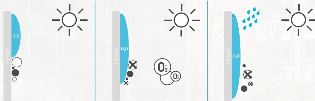
**1** The surface tension of the water is overcome. A fine film of water is formed.
