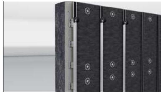
Apply joint tape on vertical bearing profiles
